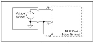
Figure 6. Connecting a Single-Ended Voltage Signal to the NI 9215 with Screw Terminal
